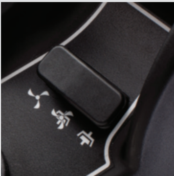
T Series tractors feature a push-button controlled power take-off for driving accessories
